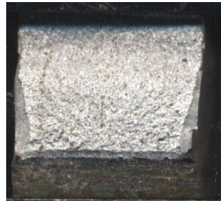
Fig. 9. Macroscopic view of the grade B27 fracture. -40°C. Hard./temper.
